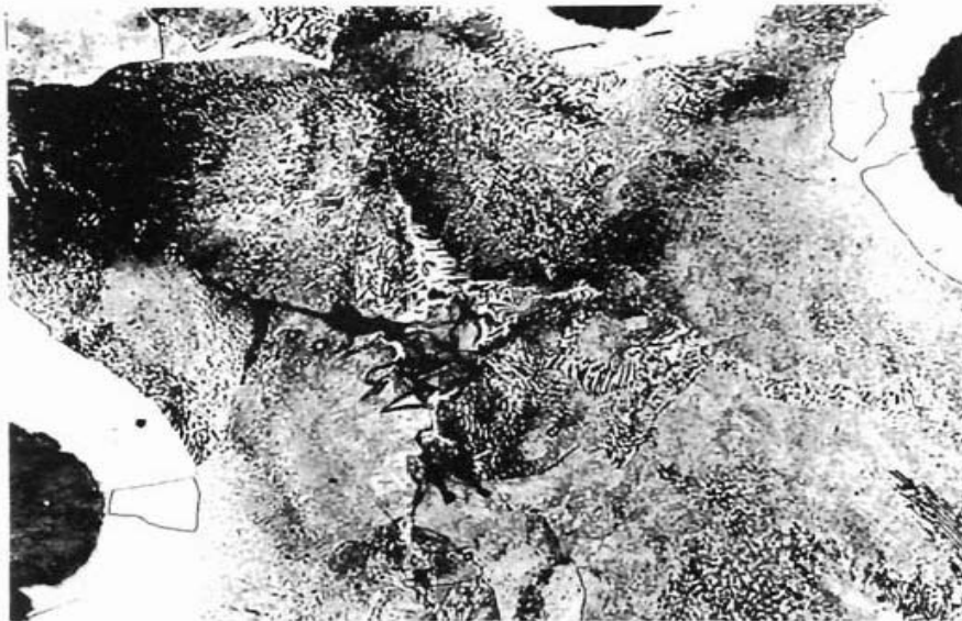
Figure 1. A 1000X photomicrograph depicting cell boundary carbides in ductile iron. (Reference is Ductile Iron Handbook , American Foundrymen's Society, 1992. p 228) Such a phase results from carbide stabilizing elements such as Mn, Cr, V, Mo, Nb and Ti segregating to the cell boundary during solidification.
